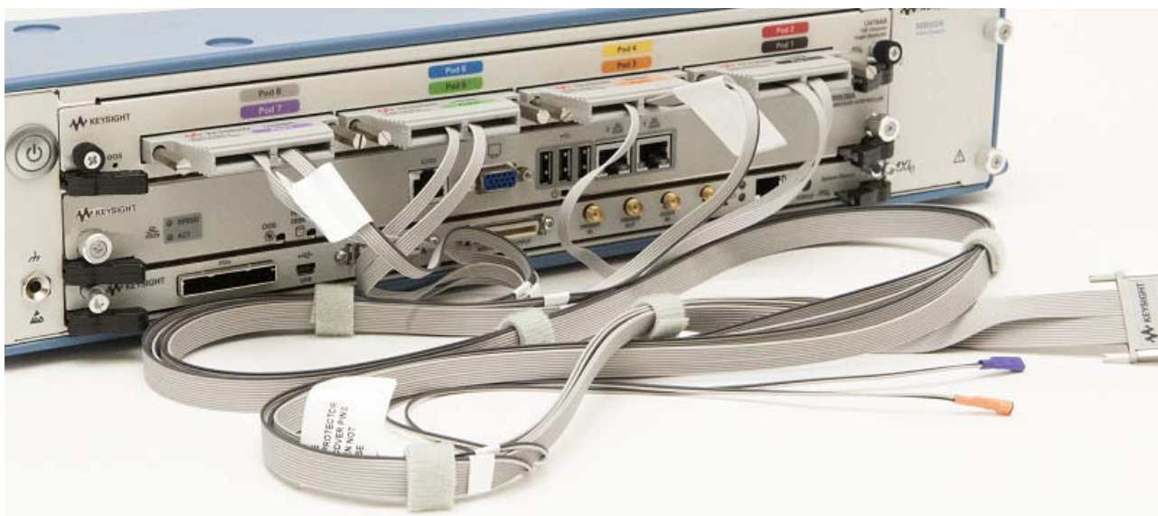
Figure 120 U4206A connected to U4164a Logic Analyzer pods
