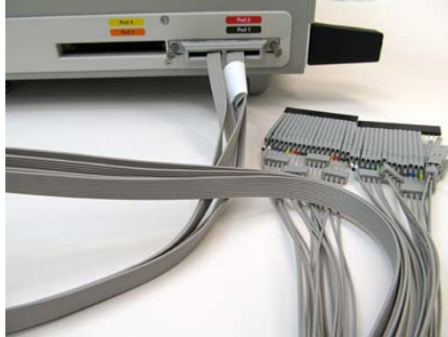
Figure 2 U4203A probe connected to a Logic Analyzer
