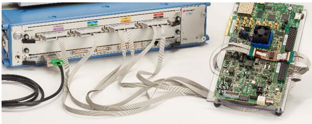
Figure 123 Sample setup for U4208A and U4209A probes
